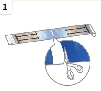
1 Cut the wallpaper a bit bigger than your door. The overhanging borders will be cut off at the end. The second strip is upside down.
