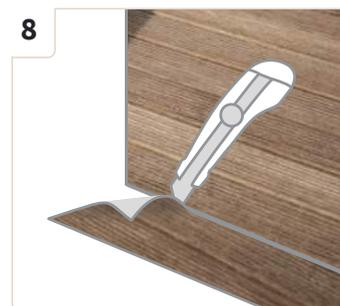
8 With a box cutter cut the overlaying edges. Ready!
