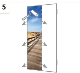
5 Flatten each strip from the upper to the lower side while pressing out the air between the wallpaper and your wall to the sides.
